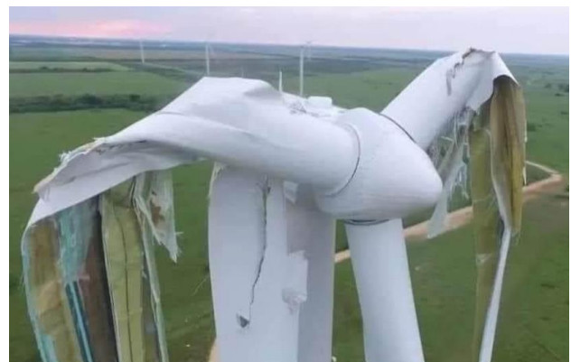
Collapse of wind turbine blades having possibly suffered structural de-bonding and buckling damage in a unit from an anonymous plant after a heavy storm.
