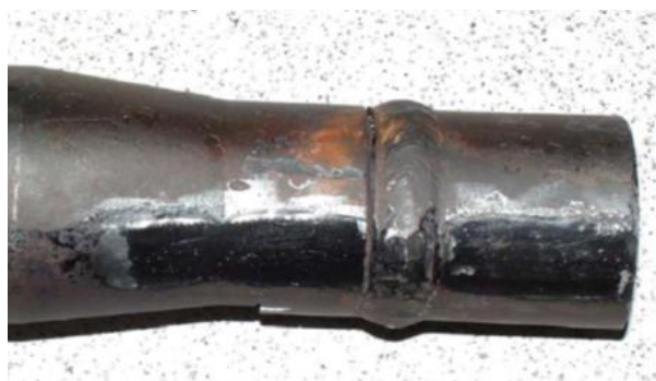
Type IV cracking on the F91 side of a weld between an F91 forged transition bottle and a T91 tube (48mm OD) taken from Ref [2].
