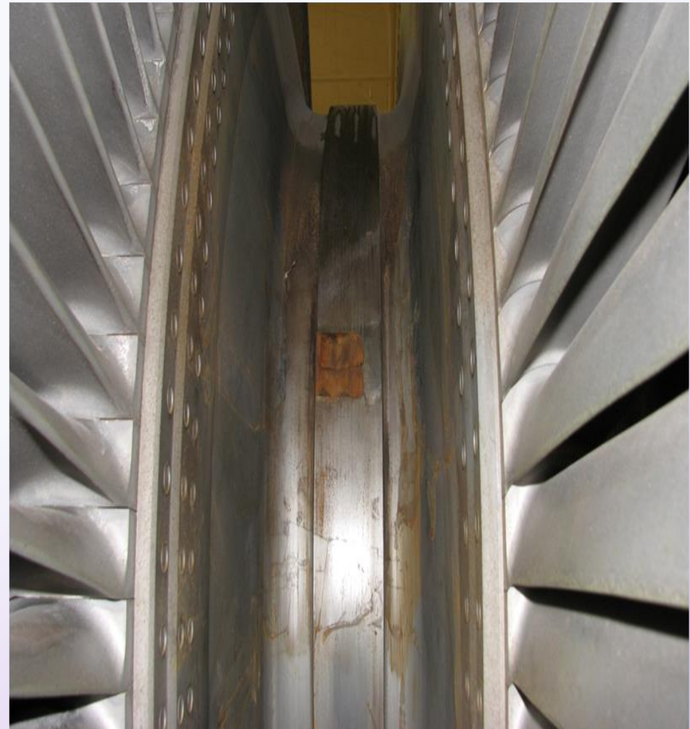
Sample cut from a rotor between two discs.
