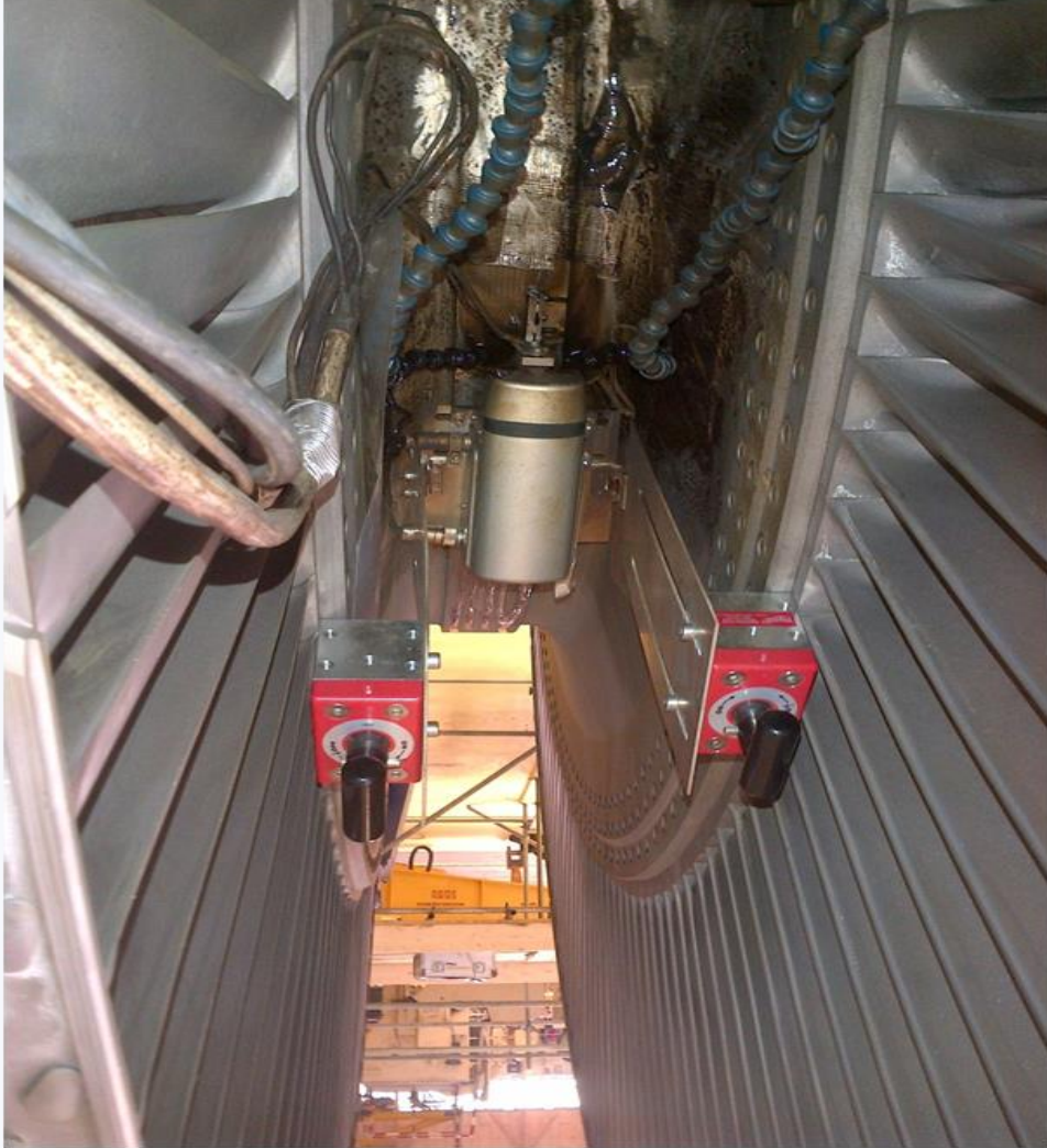
EDSE mounted between 2 discs of a rotor using magnetic mounts (red tops).
